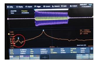
Voltage notching (phase to phase commutation short circuit)
