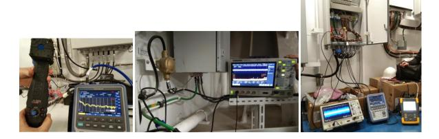
Example of fast switching AFE conductive EMI spectra and occurance of 40kHz harmonics: drive producers trade regulated 'low' harmonics/THD (DC to 3.2kHz) for 'unregulated' superharmonics and EMI.
