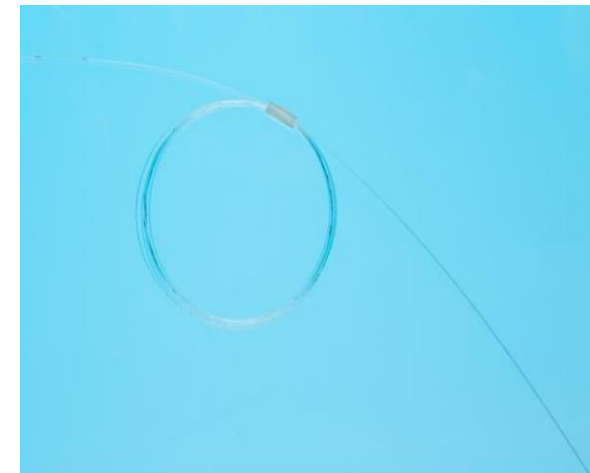
FBG Sensor in Acrylate Coated Fibre
